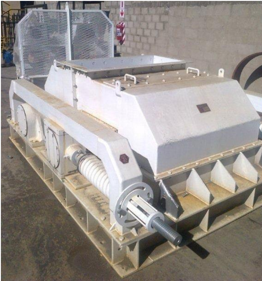
Photograph 3: BC Seam secondary crusher
