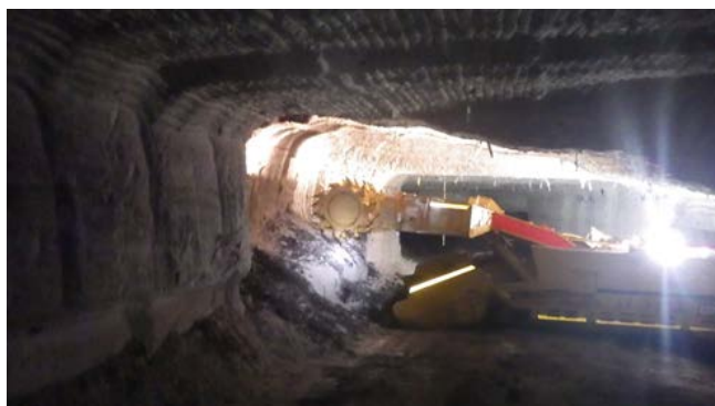
The first continuous miner section producing coal underground at the NCC operation – board and pillar operation
