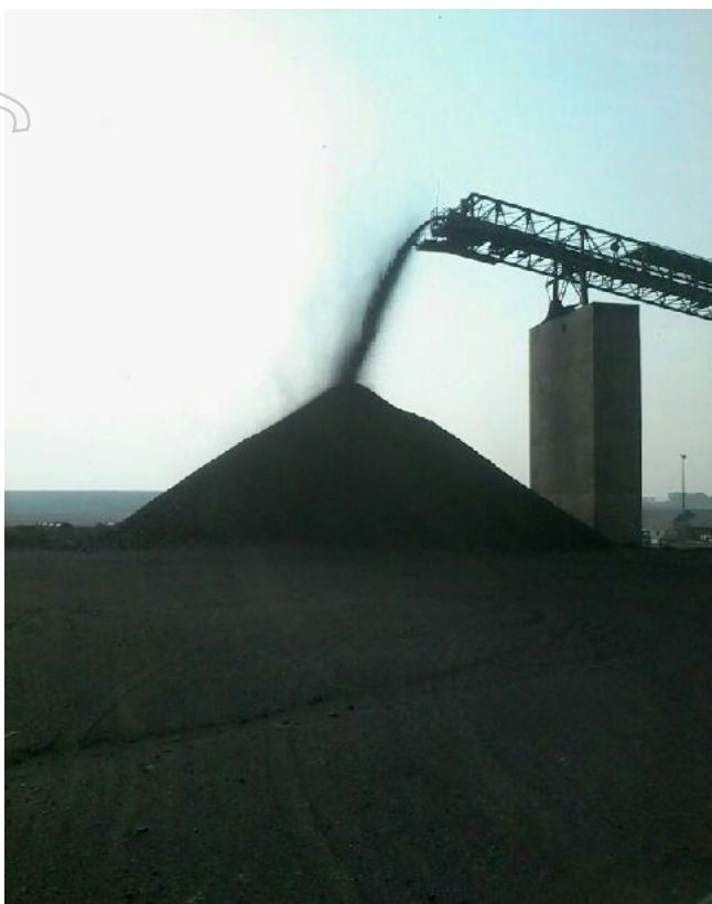
ROM Coal from underground being stockpiled for dispatch to the central Coal Handling and Processing Plant. At steady state two sections will be producing at a rate of 3,000tpd.
